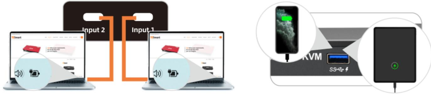
When charging using USB-A and USB-C ports, data transmission can be supported. support BC 1.2 protocol, and is able to match voltage and current automatically based on the specifications of charging devices. It makes your charging safe and avoid damage.
